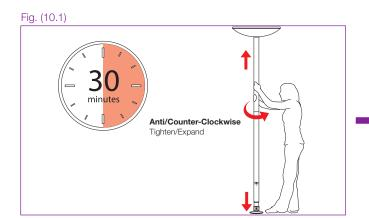
Because the XPERT Pro pole uses pressure to remain in position. The pole tightness and X-Joints should be checked regularly during use, ideally every 30 minutes.
