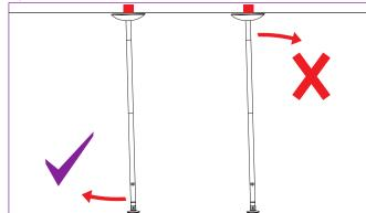
If the pole is not vertical, move the base into the required position. **DO NOT** move the Upper Dome which must be kept over the centre of the joist at all times. To move, undo the pole and reposition,
