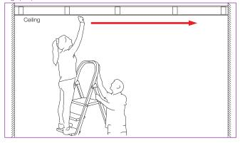
To find a Joist above your ceiling, tap across the ceiling with your knuckle until a solid sound is heard – this will be the Joist. If you keep tapping across the ceiling the sound will become hollow – the space between the Joints.
