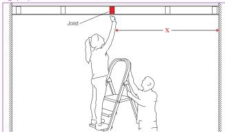
Once a Joist is located, take a position measurement from the wall for future reference. Write this measurement here: **x** =
