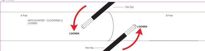
Lay the pole tubes on the floor and undo the X-Joints to disassemble the XPERT Pro. To undo the X-Joint – turn both Hex Screws **Anti/Counter Clockwise** – undo screws until there is pressure against the key.
