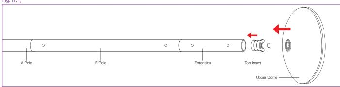
Once the A-Pole and B-Pole (and any additional extensions) are connected, insert the Top Insert into the B-Pole or last extension used, then slide the upper dome onto the top insert.
