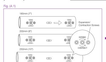
There are 3 sizes of X-Joints; 180mm (7"), 200mm (8") & 250mm (10"). The XPERT Pro is supplied with:
