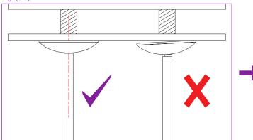
It is critical that the Upper Dome is flat against the ceiling/Joist. DO NOT expand the adjuster further until the upper dome is flat against the ceiling/Joist. If the Upper Dome is not flat, the plate could rotate, and slip or damage the ceiling.
