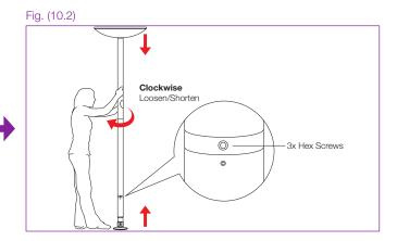
To take down the pole, ensure the X-Lock is in static/non-spinning mode and undo the 3 x Hex Adjuster Locking Screws (DO NOT completely remove the screws). Then turn the pole clockwise to contract/release the pole. Once the pole has been removed from its position, the Upper Dome can be removed.
