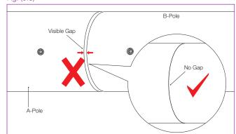
Insert a 200mm X-Joint (250mm X-Joint for 40mm and Silicone poles) into the A-Pole ensuring the keys locate into the U Slots and the expansion screws line up with the holes on the pole tubes. Next attach the B-Pole to the A-Pole with the X-Joint ensuring the Keys engage with the U Keyway Slots.
