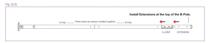
Then, as required, keep adding X-Joints and Extensions to reach your desired height – minimising the number of joints and extensions by using optional longer extensions, available from our online shop; **www.xpole.com** (first select your region, then search for 'Extensions') or local supplier.
