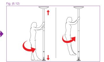
Once the pole is tight, rotate the pole until one of the three Adjuster Cover Keyhole's is in alignment with the red vertical line on the Adjuster. This will ensure that the pole is properly aligned. Failure to do so will permanently damage your pole. Now tighten the 3 Adjuster Locking Hex Screws tightly with a 5mm Hex Key to lock the A-Pole.
