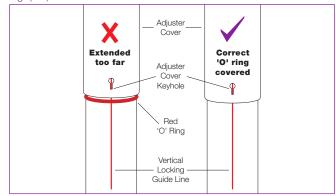
When expanding/unwinding the pole Anti/Counter-clockwise, the adjuster cover will rise. If a red 'O' ring on the adjuster is exposed, this indicates that the adjuster is over extended and you will require an additional extension to use your pole which can be purchased from our website **www.xpole.com**
