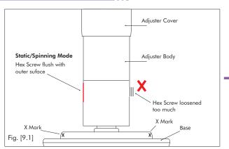
To change the pole mode from static to spinning – undo the 2 x Static/Spin Hex screws at the bottom of the pole, until they are flush with the pole - DO NOT REMOVE COMPLETELY – the pole will now spin freely.
