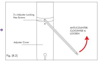
3. Now undo the 3 Adjuster Locking Hex Screws on top of the Adjuster Cover with the 5mm Hex Key - a minimum of 2 whole turns. (DO NOT completely remove the screws).
