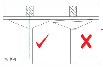
7. It is critical that the Upper Dome is flat against the ceiling/Joist. DO NOT expand the adjuster further until the upper dome is flat against the ceiling/Joist. If the Upper Dome is not flat, the plate could rotate, and slip or damage the ceiling.
