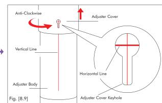
10. When expanding/unwinding the pole Anti/Counter-clockwise, the adjuster cover will rise. If a horizontal line on the adjuster is exposed in the keyhole – this indicates that the adjuster is close to 100mm. It is at 100mm when the line is below the adjuster cover. Consider buying an extension from our website www.xpole.com
