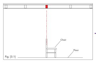
Place a chair beneath the location where you have identified your Joist OR imagine a fully assembled pole beneath this spot.
