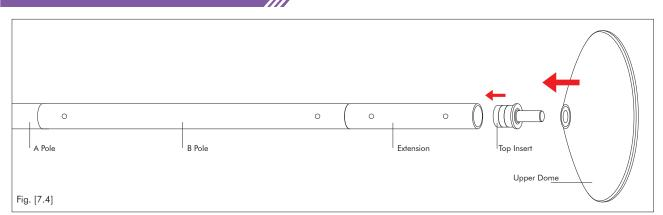
1. Once the A-Pole and B-Pole (and any additional extensions) are connected, insert the Top Insert into the B-Pole or last extension used then slide the upper dome onto the top insert.
