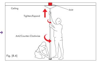
5. Once vertical, with the second person still holding the base, rotate the pole, Anti/Counter-clockwise (i.e. rotate left to right) which will expand the pole until it touches the ceiling.
