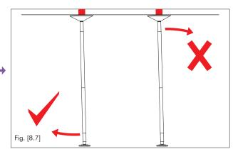
8. If the pole is not vertical, move the base in the required direction. DO NOT move the Upper Dome which must be kept over the centre of the Joist at all times.
