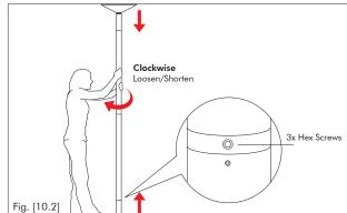
2. To take down the pole, undo the 3 x Hex Adjuster Locking Screws (DO NOT completely remove the screws). Then turn the pole clockwise to contract/ release the pole. Once the pole has been removed from its position, the Upper Dome & Base can be removed.
