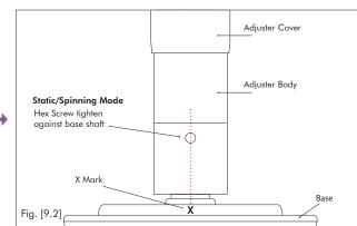
2. To return to static, rotate the pole till one of the hex screws is in alignment with the 'X' on the base plate and FULLY tighten. Whilst tightening, gently rotate the pole back and forth to help seat the screw. Now fully tighten the other screw.
