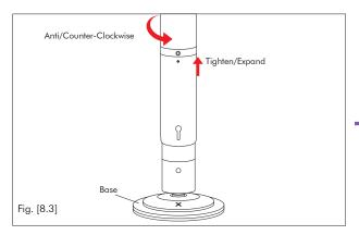
4. Pole Expansion: Rotating the main pole tube from left to the right (Anti/Counter-Clockwise) will Expand/Tighten the Pole. Rotating the pole tube from right to the left (Clockwise) will Shorten/Loosen the Pole.
