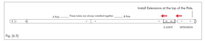
5. Then, as required, keep adding X-Joints and Extensions to reach your desired height – minimising the number of Joints and tubes by using optional longer extensions (available from our online shop; www.xpole.com - first select your region, then search for 'Extensions') where possible.
