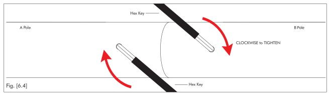
4. It is important to tighten the screws progressively – alternating between the screws, tightening Clockwise. This will ensure the pressure is equalised within the pole tubes.
