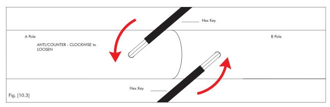
3. Lay the pole tubes on the floor and undo the X-Joints to disassemble the XPERT. To undo the X-Joint – turn both Hex Screws **Anti/Counter Clockwise** – undo screws until there is pressure against the key.
