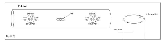
1. At the centre of the X-Joint are 2 x Keys. These Keys slide into the corresponding U Keyway slots in the pole tube.
