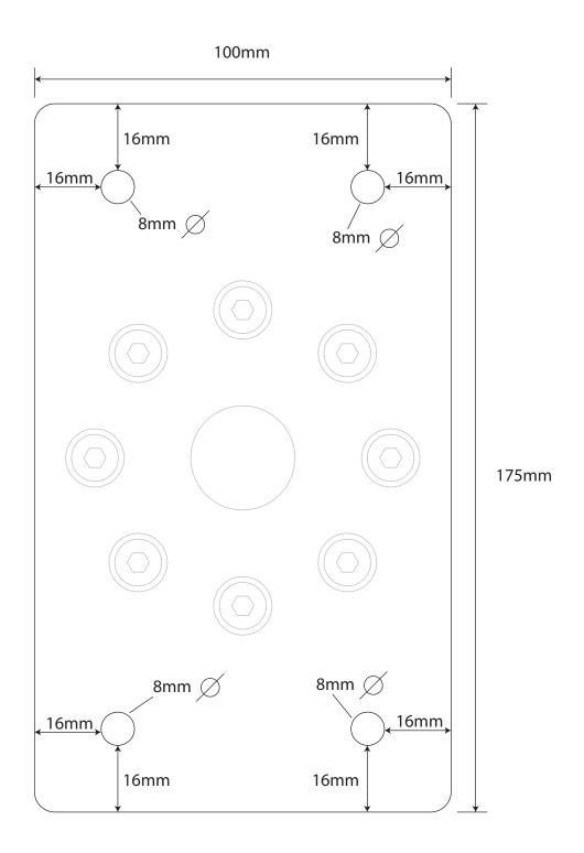
Use 8mm Screws to mount the plate\* The length of screw differs depending on where the plate is mounted. (Wood Beam, Concrete Ceiling)
